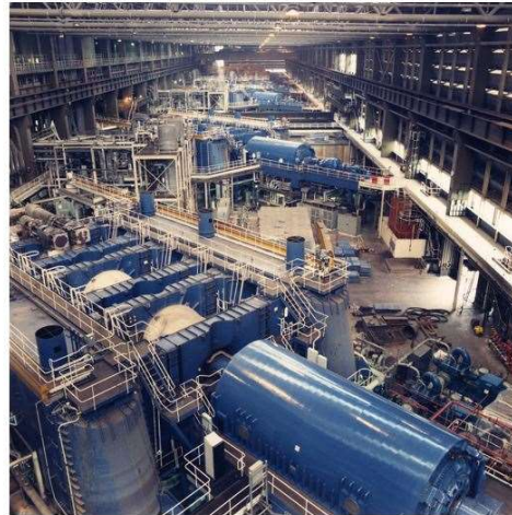
British Steel Corporation has supplied many complete rotor sets — seventy four forgings to date — for 660 MW turbine generators. This unit is being test assembled at the Newcastle Works of C A Parsons &
